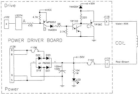
The microprocessor toggles the output of the 74LS374. When point "A" is low, point "B", the collector of the 2N5401 transistor, is high. A high at point "B" causes point "C", the collector of the TIP102 transistor and point "D", the emitter of the TIP36C transistor, to drop low. When point "D" is low, the coil is grounded through the transistor and turns on. The coil shuts off when point "A" toggles high.
