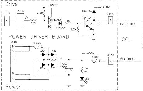
The microprocessor toggles the output of the 74LS374. When point "A" is low, point "B", the collector of the 2N5401 transistor, is high. A high at point "B" turns on the TIP102 transistor and causes point "C" to drop low. When point "C" is low the coil is grounded through the transistor and turns on. The coil shuts off when point "A" toggles high.
